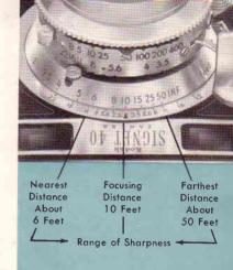
Distances are measured from the film plane to the subject. The film plane indicator — on the top of the camera, locates the film plane.
