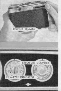
7 Turn the EXPOSURE COUNTER dial in the direction of the arrow until the index mark is opposite the red 20 for a 20-exposure magazine—the red 0 for a 36-exposure magazine. The counter will move a mark for each picture taken. It will always show the number of exposures remaining on the film. The exposure counter will not work unless there is film in the camera.
