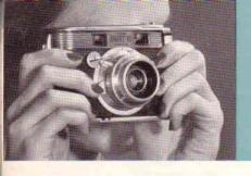
You adjust focus by moving the focusing lever with your finger. The rangefinder images are tinted in contrasting colors for easy, accurate focusing.
